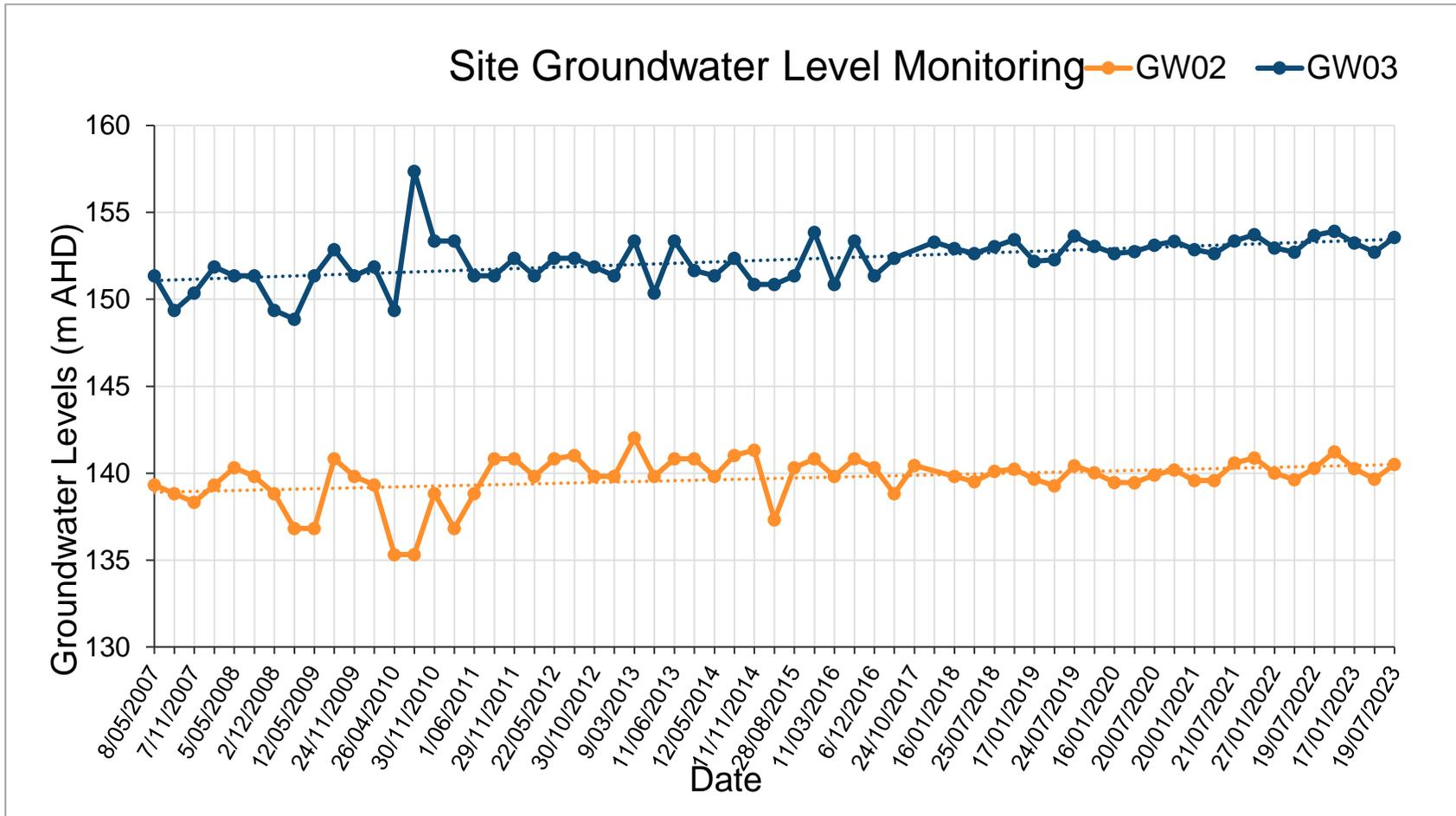
Figure 2. Groundwater levels in m AHD for GW02 and GW03 locations.
