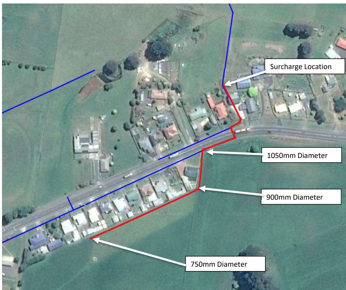
Figure 2 Mitigation Option 1B Pipe east along property boundary the north across highway.
