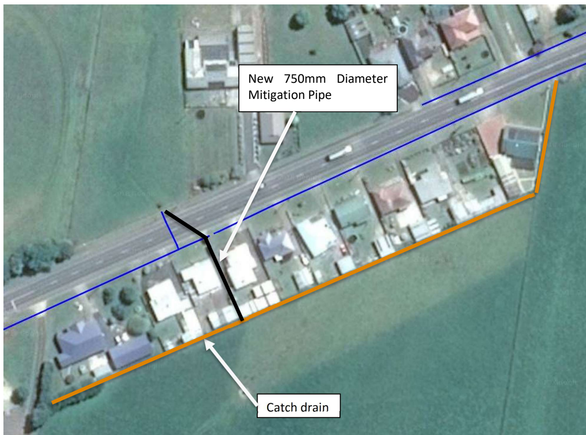
Figure 2 Mitigation Option 1A Pipe Under private property discharging northern side of Highway into Cooee Creek
